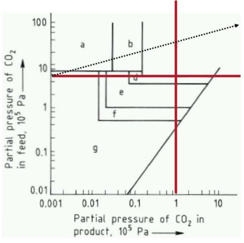
Trade-off at  $P_{CO2} \sim 5$  bara between solvent loading/recirculation (lean vs. rich) and equipment sizing
