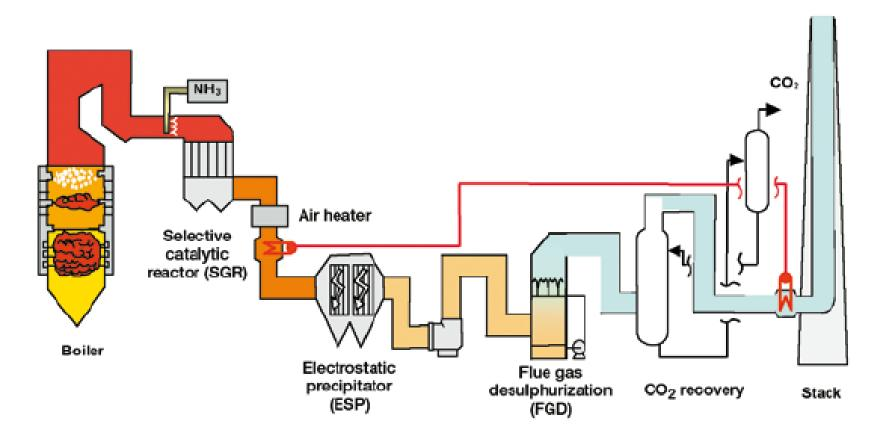
• In post-combustion capture system, CO<sub>2</sub> captured from flue gases produced by combustion of fossil fuels and biomass
