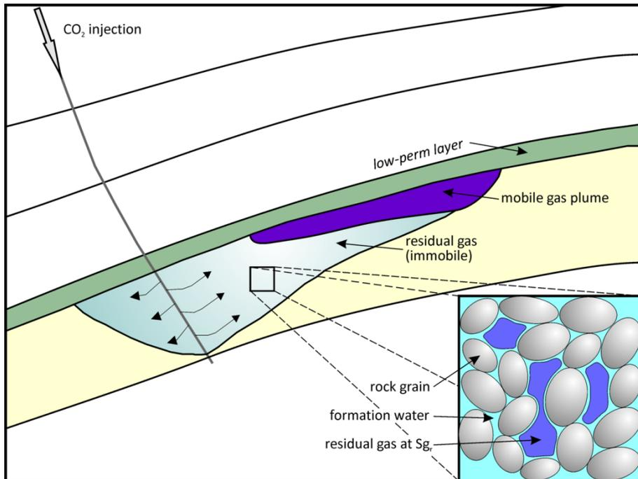
Schematic of trail of residual CO<sub>2</sub> that is left behind because of snap-off as the plume migrates upwards during post-injection period (modified from Juanes et al. 2006 and CGSS 2010)
