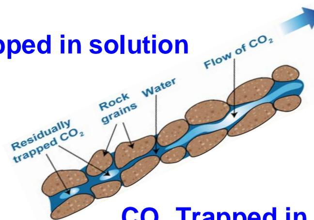
CO<sub>2</sub> Trapped in rock pores as Residual Saturation
