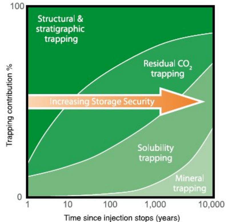
Figure 5.9 Storage security depends on a combination of physical and geochemical trapping. Over time, the physical process of residual CO<sub>2</sub> trapping and geochemical processes of solubility trapping and mineral trapping increase. IPCC SRCCS 2005
