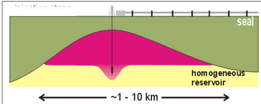
Conventional trap – may be a depleted field or a “dry” structure
